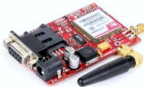
Figure 17 GSM Module.
