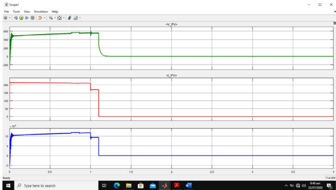
Figure 3.4: Power, Voltage and Current generated by solar arrays
