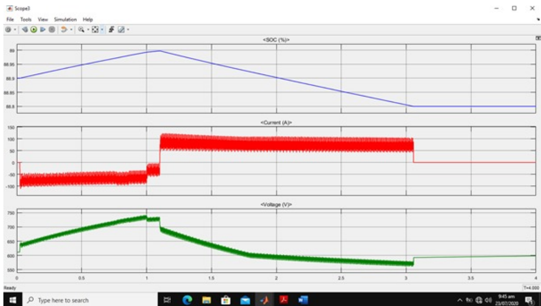
Figure 4.4: Battery SOC Charging Discharging, load current and voltage, Load at 3.1 sec load shifted on diesel generator.
