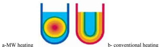
Fig. 1. Microwave heating and conventional heat dissipation
