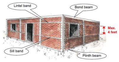
Fig.3. Increasing the stability of a building against earthquake [11]
