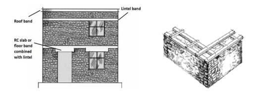
Fig. 1. Reinforced concrete and timber bands [10]
