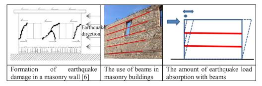
'In some regions of the world, timber or brick bands are used to enhance the wall stability in both uncoursed random rubble and semi-dressed masonry. This is a traditional practice in some parts of Nepal, İndia, Pakistan, Turkey and Greece' [10]. Recommended use of timber and reinforced concrete bands (hatils) in Turkish stone masonry are shown in the figure 1.
