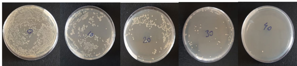
Fig. 8 The antibacterial effect changes with the increase in the bacteriostatic time on the AC/Ag composite
