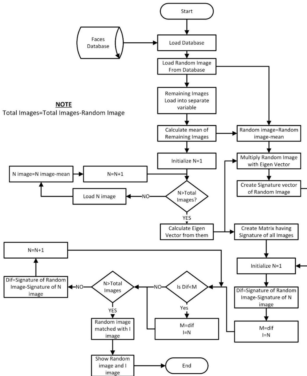
**Figure 34:** Flow Chart of Face Recognition Algorithm
