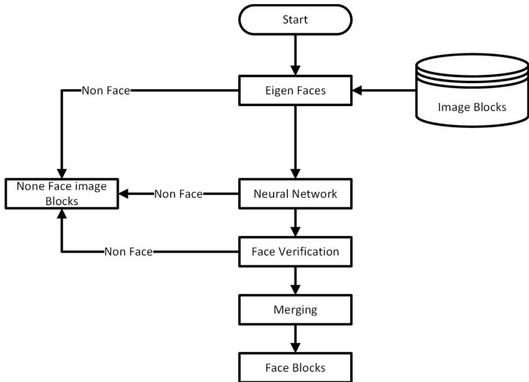
**Figure 18:** Algorithm of Face Detection Using Eigen face and Neural Network
