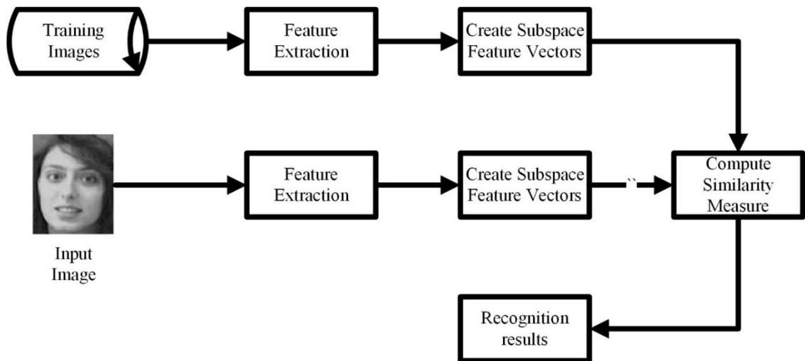
**Figure 21:** Face Recognition using Layered Linear Discriminant Analysis
