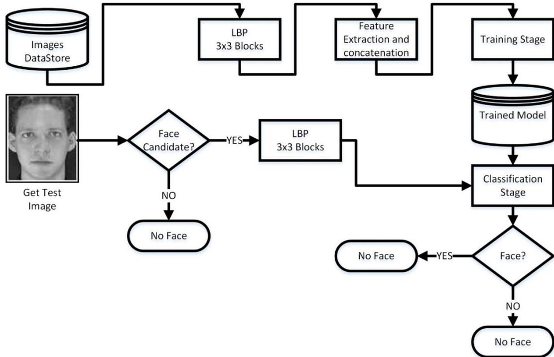
**Figure 24:** Face Recognition using LBP Method
