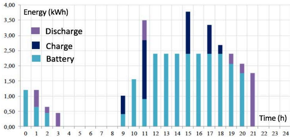
Figure 29 Daily Change of Battery Charge and Discharge Status in Optimally Distributed Load Status in Pure PV System
