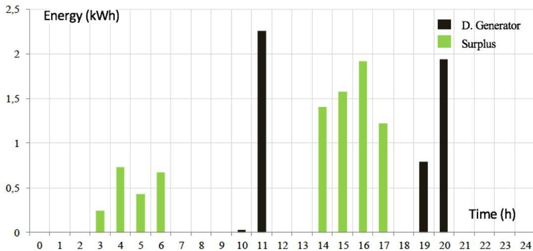
Figure 24 Daily Change of Energy Generated by Extra and Diesel Generators in Pure Wind Turbine System
