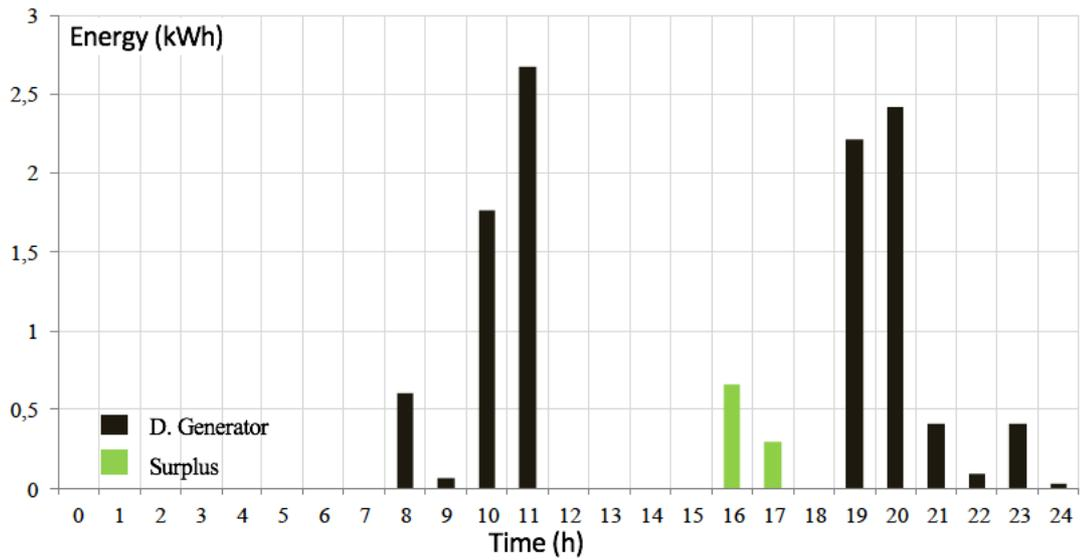
Figure 27 Daily Change in Excess and Diesel Generators Produced in Wind-PV Hybrid System
