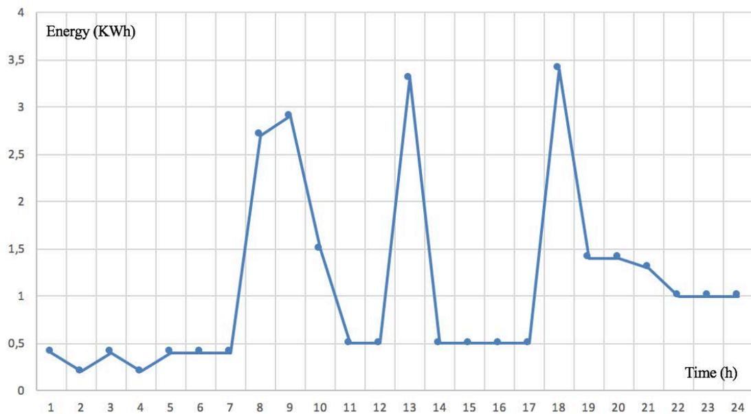
Figure 10 Load Profile for Typical Residential Home Load
