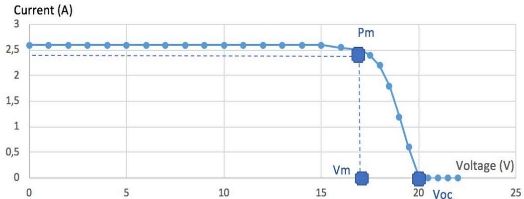
Figure 7 Characteristics of PV Module
