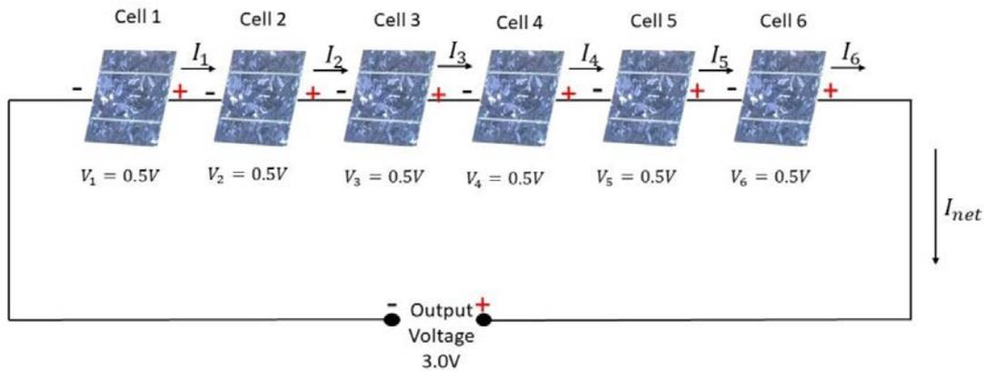
Figure 6 PV module Connected Series
