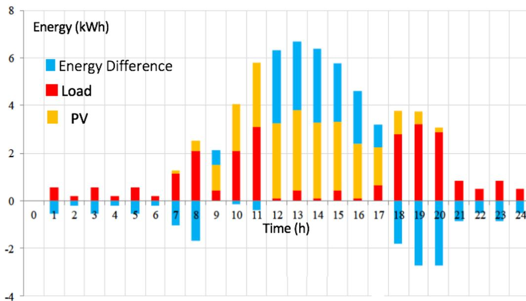
Figure 19 Daily basis of total power generation and consumption in the optimally designed PV system
