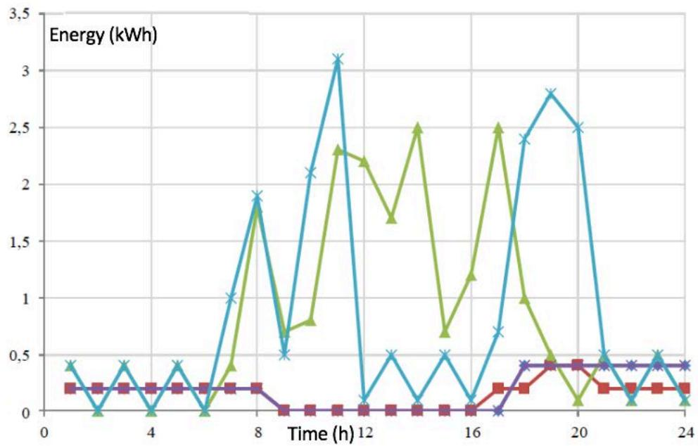
Figure 39 Daily Change of Energy Consumption of Controlled and Uncontrolled Loads in Planned-Unplanned Load Distribution in Wind-PV System
