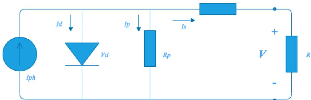
Figure 5 Single Equivalent Circuit Model of PV Cell
