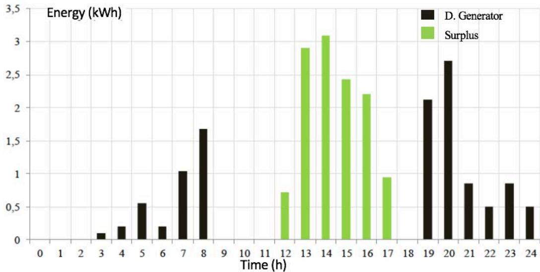
Figure 21 Time slots of a diesel generator use in the optimally designed PV system
