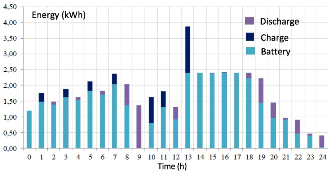
Figure 35 Daily Change of Battery Charge and Discharge Status According to Optimally Distributed Load Status in 9 PV Panels and 1 kW wind turbine System
