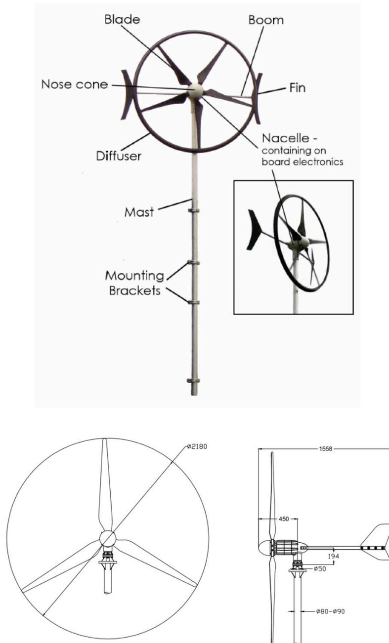
Figure 2 Structure of rooftop wind turbine
