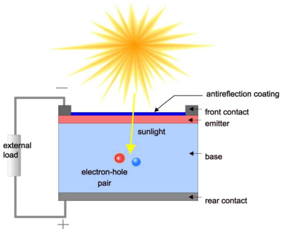
Figure 4 Basic Operation of PV Cell
