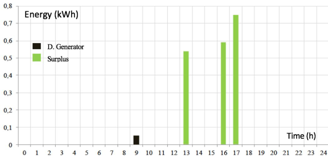
Figure 36: Daily Change of Energy Generated by Extra Diesel Generators and 9 PV Panels and 1 kW wind turbine System According to the Load Distribution
