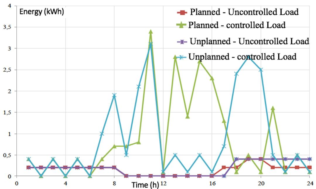
Figure 37 Daily Change of Energy Consumption of Controlled and Uncontrolled Loads in Planned-Unplanned Load Distribution in Pure PV System
