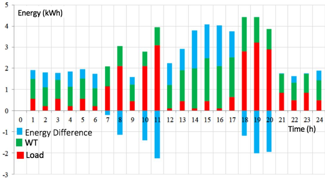
Figure 22 Daily Change of Energy Produced and Demanded with 2 pieces 1 kW wind turbine
