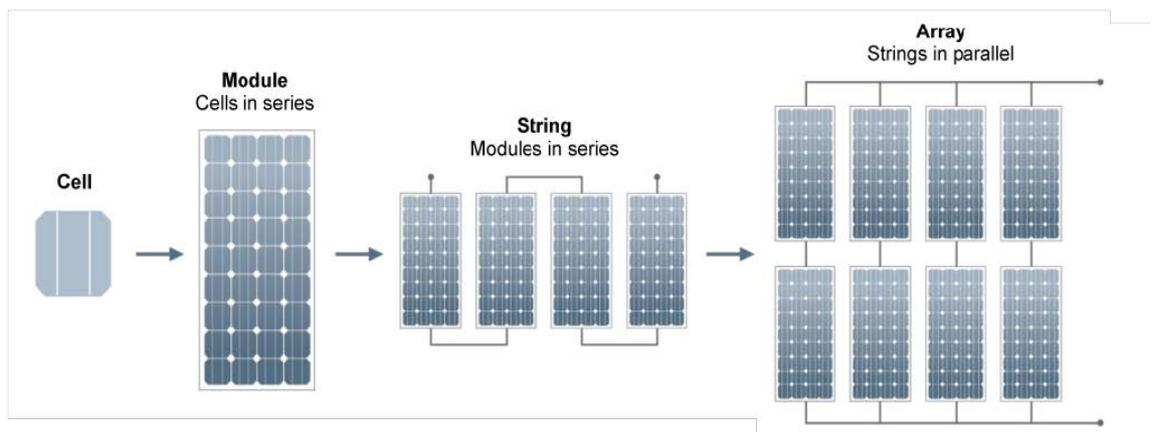
Figure 9 PV System General Layout
