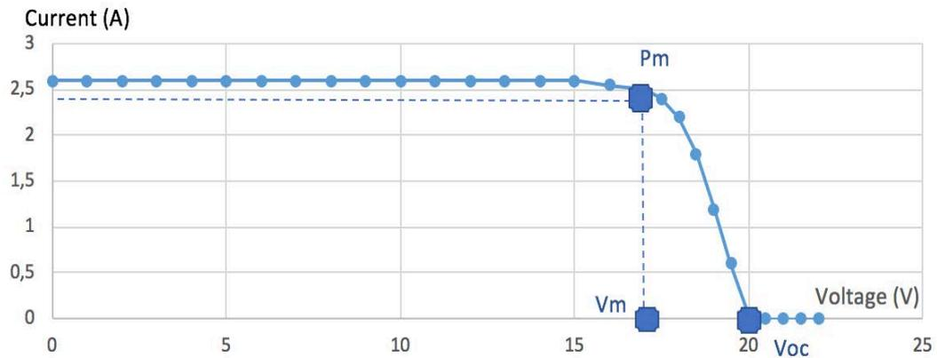
Figure 7 Characteristics of PV Module
