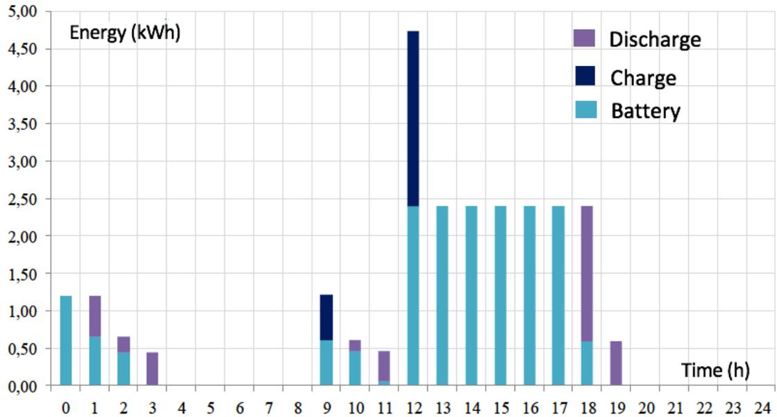
Figure 20 Daily Change of Battery Charge and Discharge Status in Pure PV System
