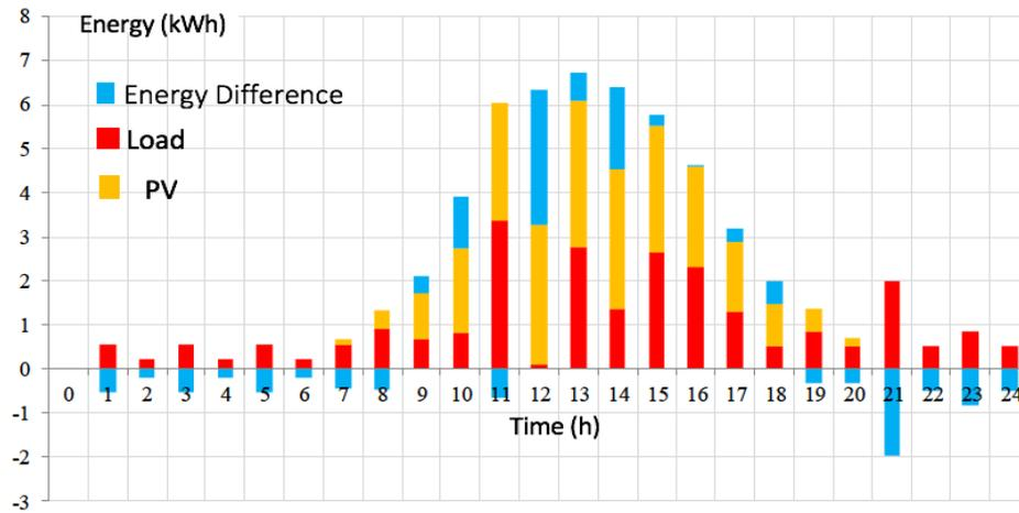
Figure 28 Daily Variation of Produced, Demanded and Difference Energy Quantities According to the Load Distributed State in Optimally Distributed PV System
