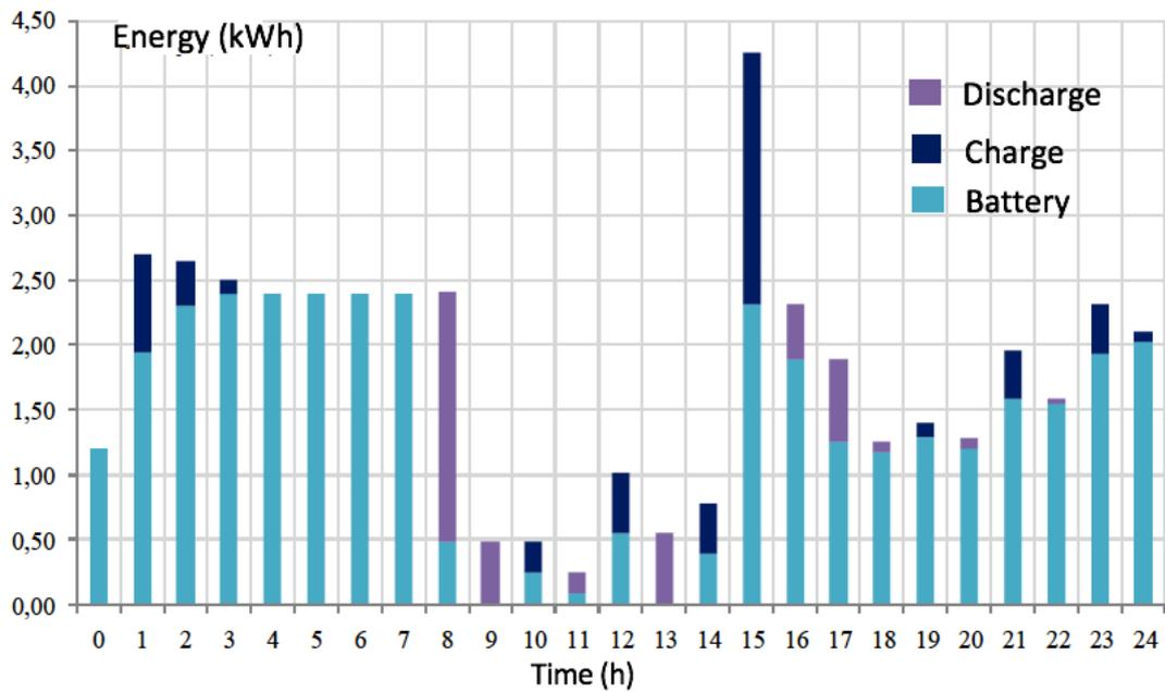
Figure 32 Daily Change of Battery Charge and Discharge Status According to the Load Distribution in the Most Optimally Distributed State in 2 pcs 1 kW wind turbine System
