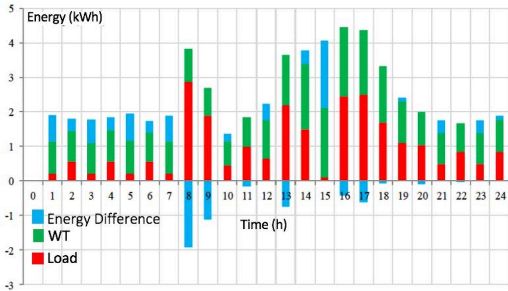
Figure 31 Daily Change of the Energy Difference Produced and Demanded According to the Load Distributed in the Optimally Distributed Load Condition in 2 Piece 1 kW wind turbine System
