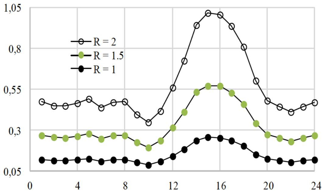
Figure 17 Variation of Power Generated at Different Wing Lengths
