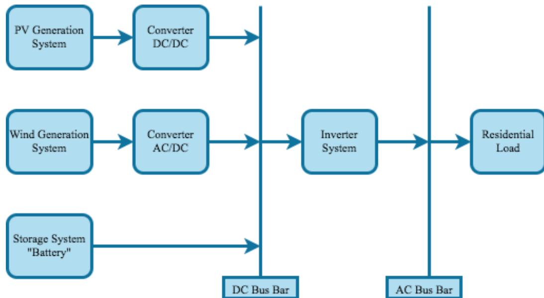
Figure 1 Hybrid System Block Diagram
