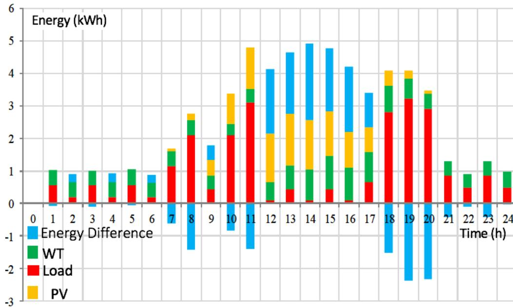
Figure 25 Daily Variation of Generated, Demanded and Difference Energy Amounts in Wind-PV Hybrid System
