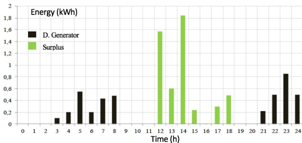
Figure 30 Surplus Based on Optimally Distributed Load Status in Pure PV System and Diesel Generator Produced By Daily Exchange
