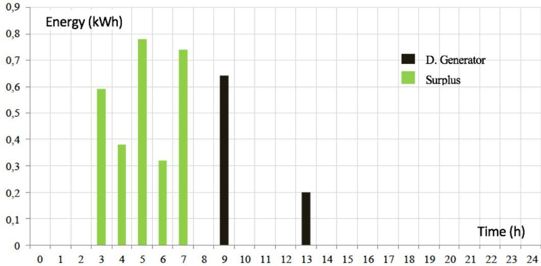
Figure 33 Daily Change of Energy Produced by 2 pieces of 1 kW wind turbine and Diesel Generators according to the most appropriately distributed load status
