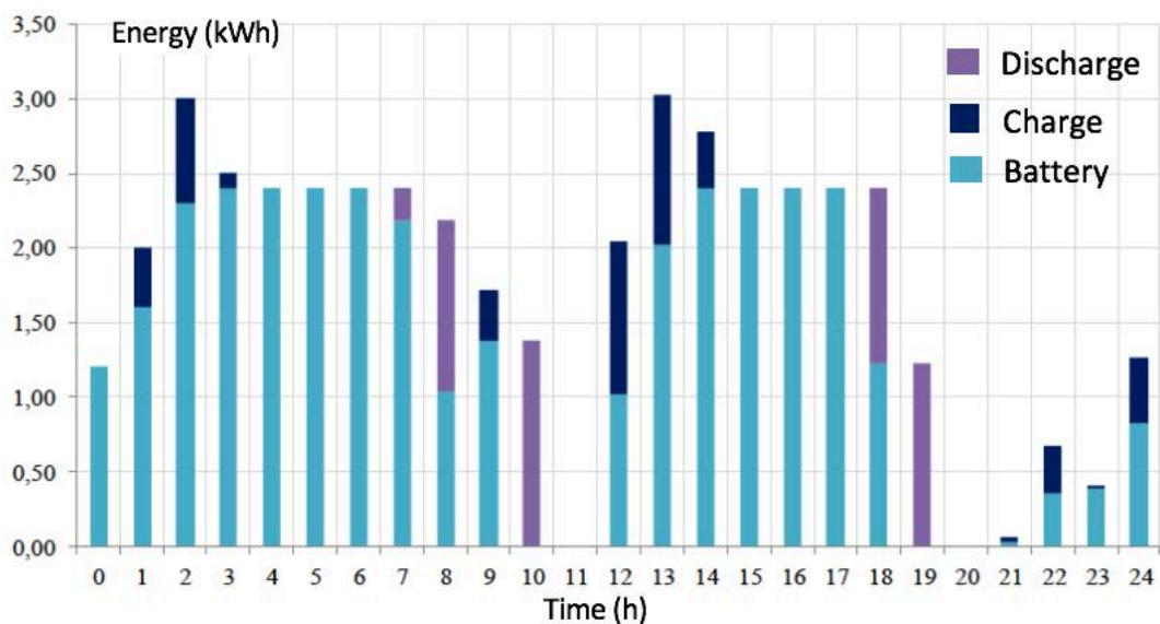
Figure 23 Daily Change of Battery Charge and Discharge Status in 2 pieces 1kW Wind Turbine Powered System
