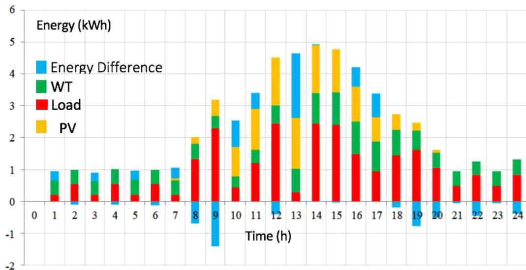
Figure 34 Daily Change of Energy and Energy Difference Produced and Demanded According to the Optimally Distributed Load Condition in 9 PV Panels and 1 kW wind turbine System
