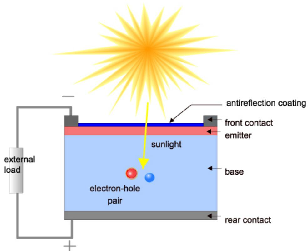
Figure 4 Basic Operation of PV Cell
