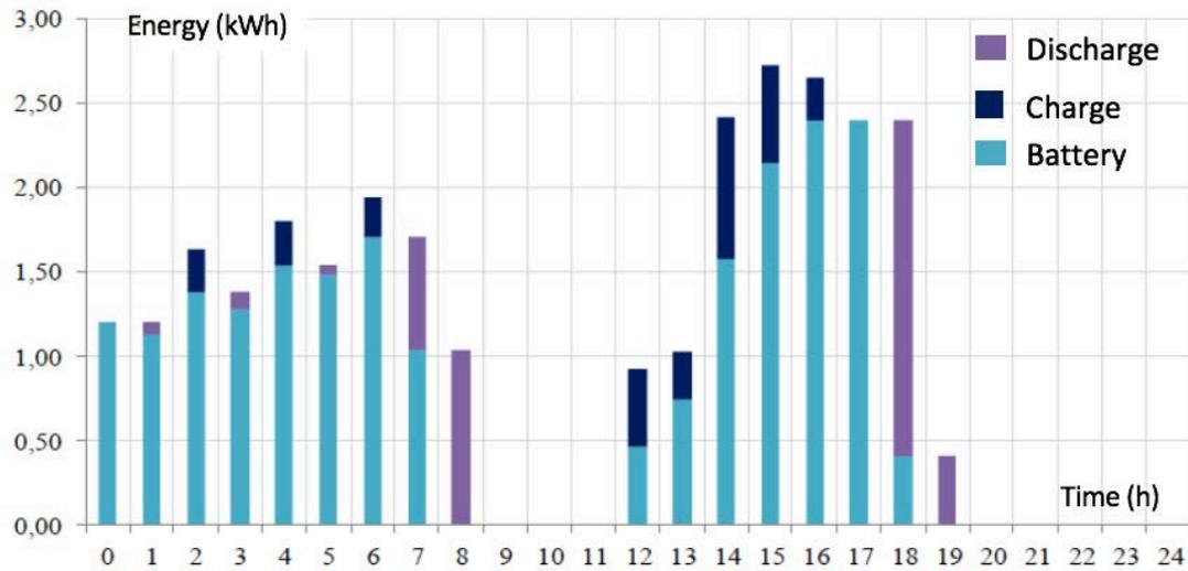
Figure 26 Daily Change of Battery Charge and Discharge Status in WIND-PV Hybrid System
