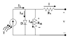
Figure 2. Photodiode equivalent circuit.
