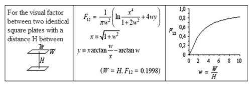
Figure 3. High vision factor for TPV applications in iron and steel industry [4, 19].
