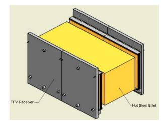
Figure 5. Four planar TPV modules placed on two layers of steel [20].
