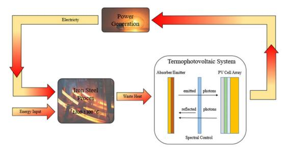
Figure 4. Energy recycling by TPV application in the iron and steel sector.
