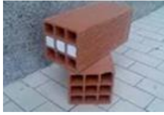
Figure 22 Perforated Bricks: It Is A Brick With Gaps in It. These Gaps Contain the Type of Insulating Cork [NAGHAM HAIDER, (2021)].
