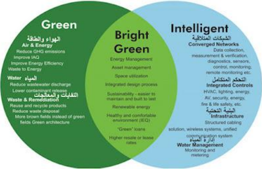
Figure 55 Combine smart buildings and green buildings to achieve a smart green building [MONA AL-ADAWY, (2022)].
