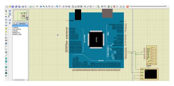
Figure 19 Simulation of Arduino Mega with GSM Module.
