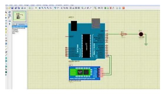
Figure 20 Simulation of Arduino UNO with Bluetooth Module.
