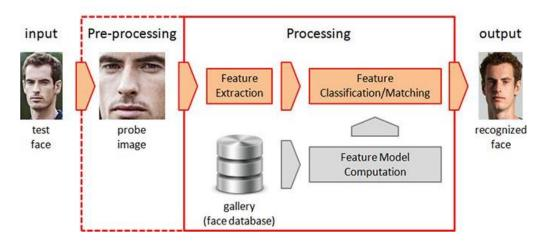
Figure 11 Image Processing Diagram.
