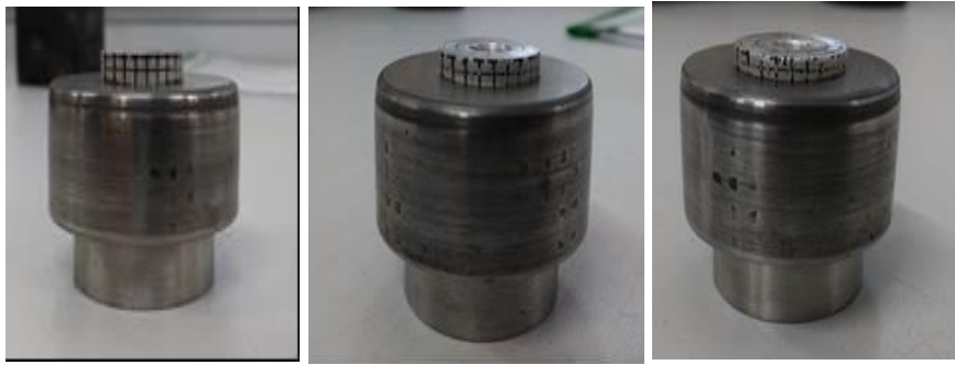
Figure 5: Side grid photos of the ring specimen.
