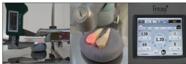
Figure 1. Preparation of Er:YAG Laser Group Specimens
