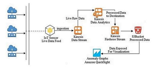
Figure I Architecture used for anomaly detection and performance testing.
