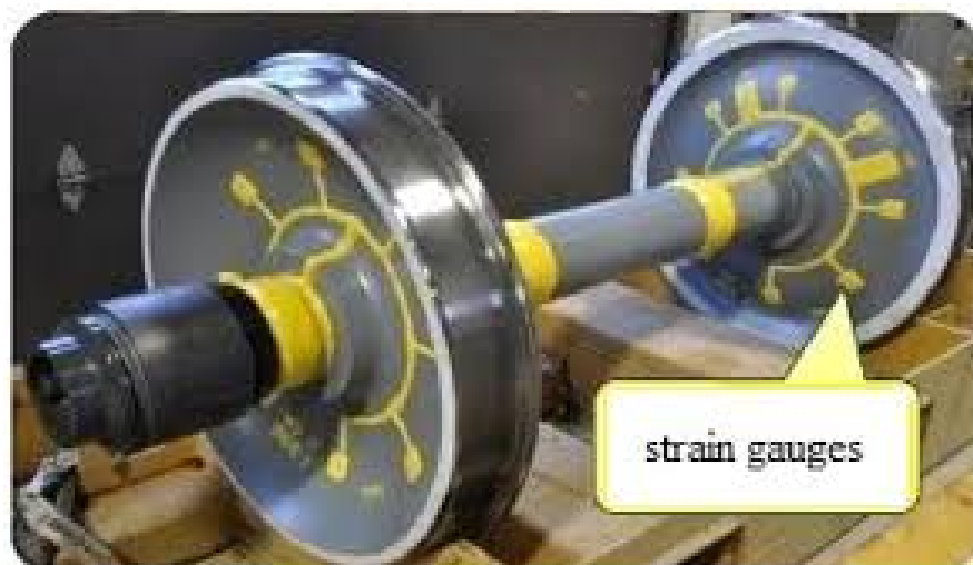
Figure 31: Instrumented railway wheel set (Ngigi, 2012)
