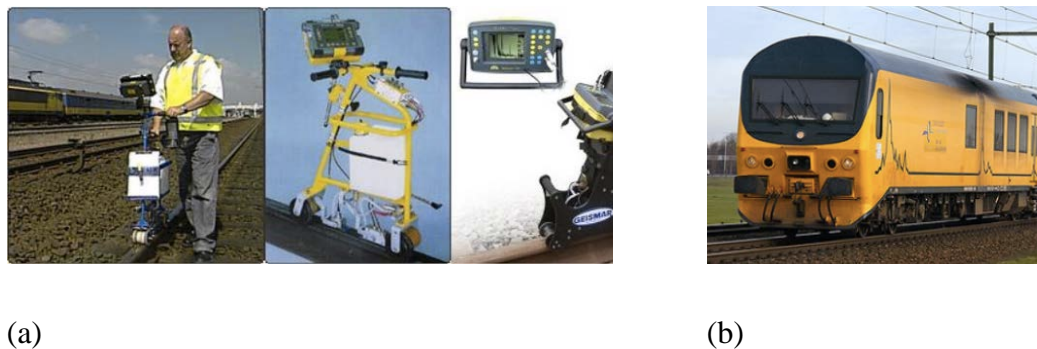
Figure 34: Ultrasonic measurement, (a) hand-held devices: euraiscout SPG 2, MT95, and geismar SIRIUS, (b) euraiscout UST96 ultrasonic train (Simões, 2008).
