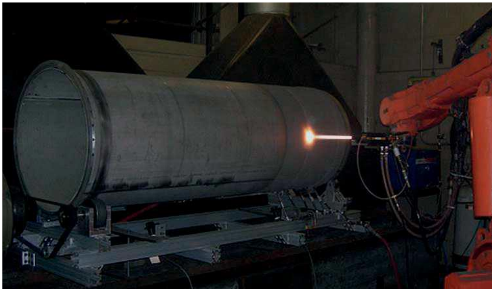
Figure 51 High Velocity Oxy-Fuel (HVOF) process is used to coat a container with SAM1651 amorphous metal with quality assurance monitoring the thickness and roughness of BMG coating
