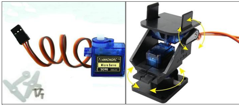
Figure 9 SG90 micro servo (left) and pan/tilt kit (right)
