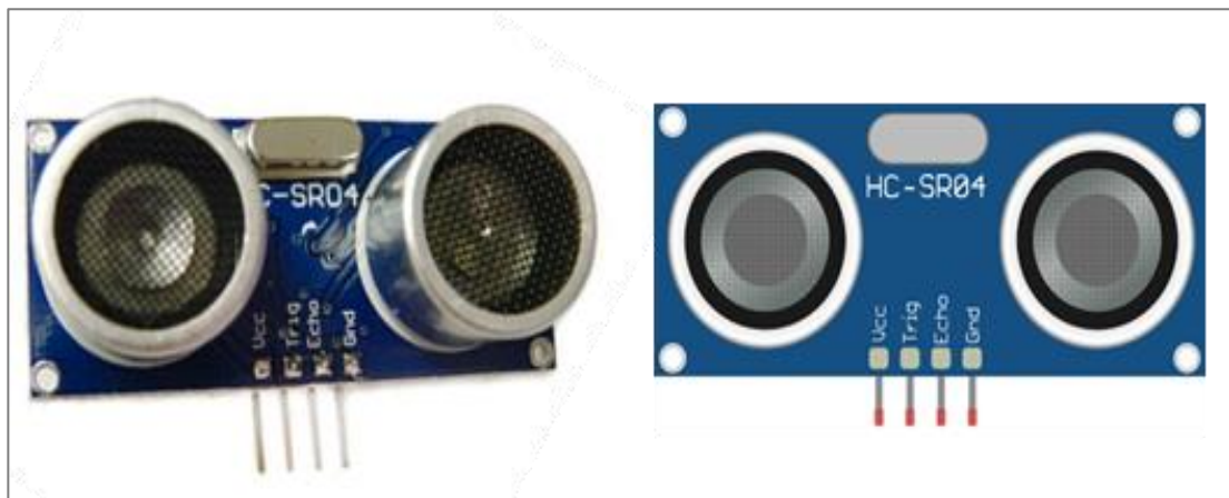
Figure 5 Ultra-sonic sensor HC-SR04 board actual (left) drawn (right)
