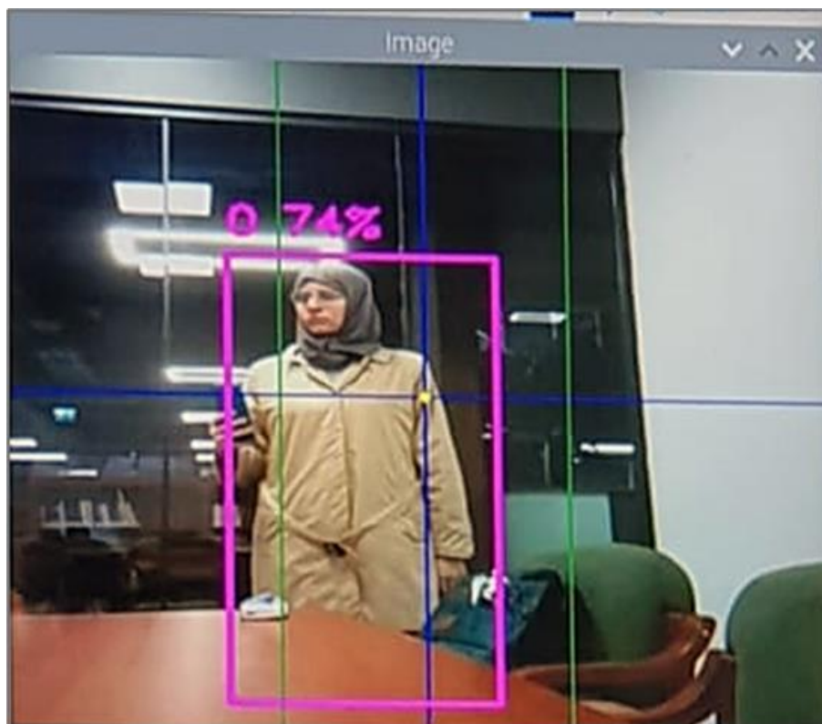
Figure 28 Clear execution of software that shows boundaries of tolerance, center of frame and center of object
