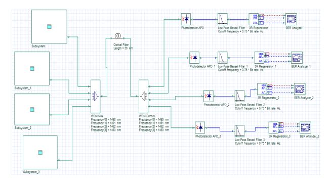
Figure 4. 4: Simulation of WDM PON
