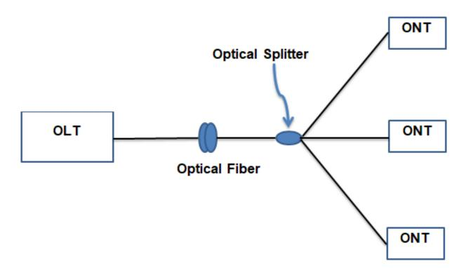
Figure 2. 5: Passive Optical Network
