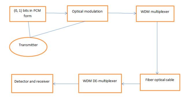
Figure 4. 3: Uni-directional WDM PON Flow Chart
