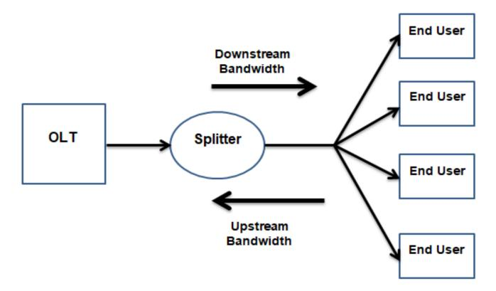
Figure 2. 7: Gigabit Passive Optical Network
