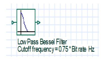
Figure 4. 16: Low Pass Bessel Filter
