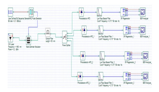
Figure 4. 2: Simulation of TDM PON
