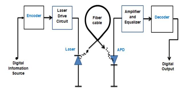
Figure 2. 3: Digital of Fiber Optic Communication System
