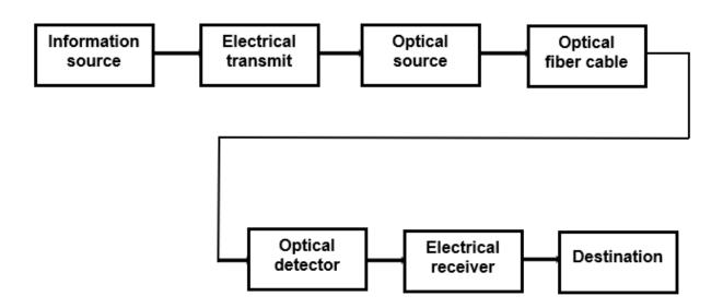
Figure 2. 2: Fiber Optic of Communication System
