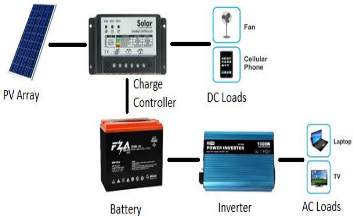
Figure 2. 17 : OFF-Grid Photovoltaic System
