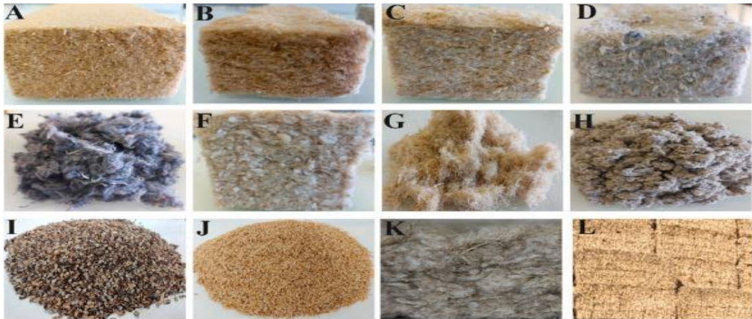
Figure 14: Several biomass-based insulating materials and products: a) wood hardboards, b) wood medium-density fiberboard, c) hemp panel, d) cellulose wadding panel, e) recycled textiles in loose-fill, f) mixed fibers (cotton/flax/hemp) panel, g) hemp fibers, h) cellulose wadding in loose-fill, i) buckwheat husks, j) millet husks, k) flax panel, l) wheat straw bales (Rabbat et al., 2022).
