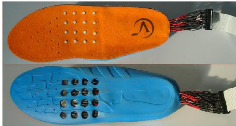
**Figure: 3 showing prototype of shoe-integrated tactile display (Velázquez, Bazán et al. 2012)**
