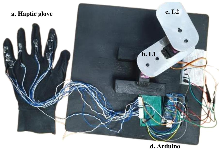
**Figure: 7 showing complete prototype system**
