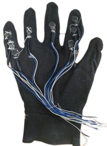
**Figure: 6 showing the prototype of the Haptic glove**
