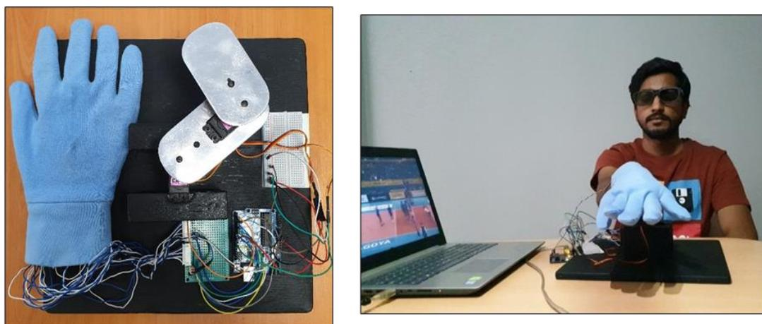
**Figure: 11** On the right, you can see the finished system. The person touches the robotic arm with his hand. It directs the hand of the user to the appropriate location
