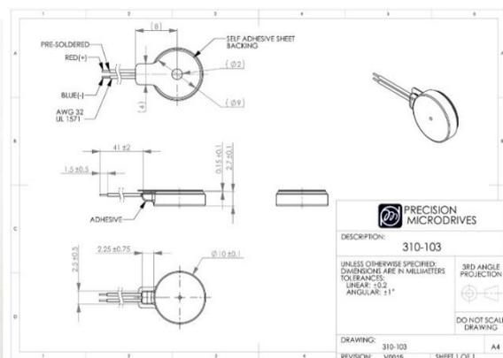
**Figure: 15 showing dimensional specification of shaftless vibration motor**
