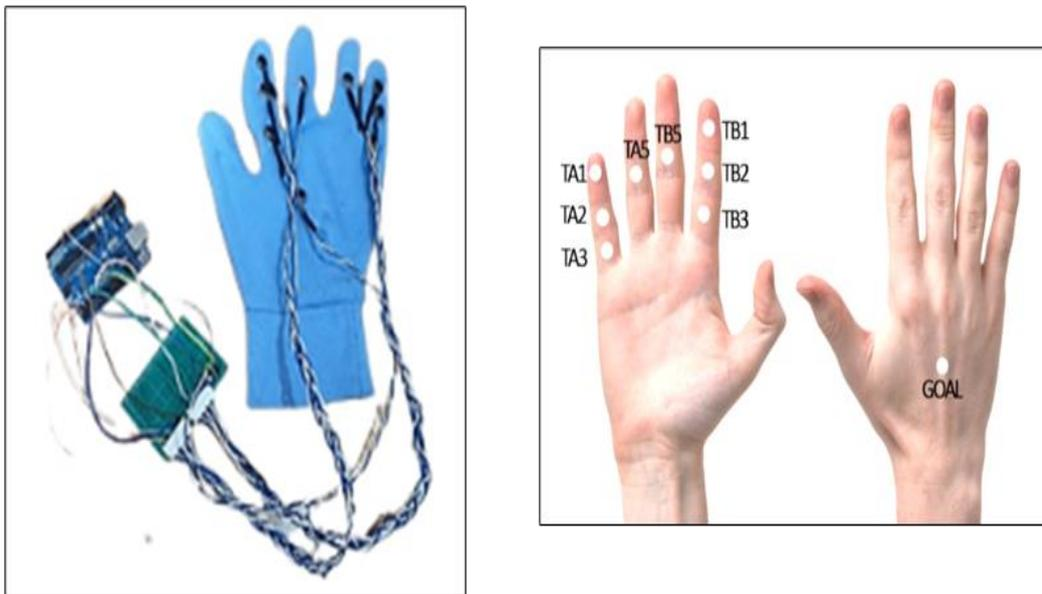
**Figure: 9 showing the position of motors incorporated in haptic glove**
