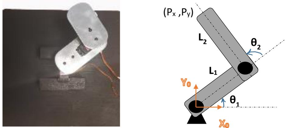
Figure: 8 showing the robotic arm, which is made up of two servomotors and two aluminum links.
